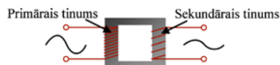
10.34. att. Pazeminošais transformators
